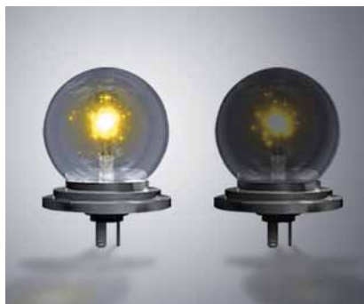
New filament bulb (left) and old blacken filament bulb (right).
