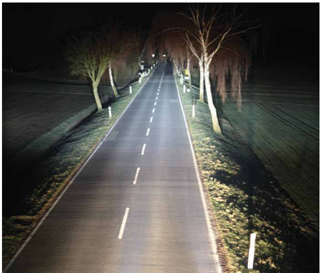
Typical light distribution and colour temperature of a light beam with HID bulb.
